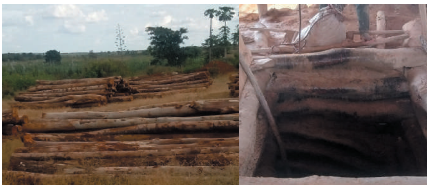
Picture 7.4: Tree logs to be used in reinforcing pits (left) and a mine pit reinforced with logs (right) observed in Geita
